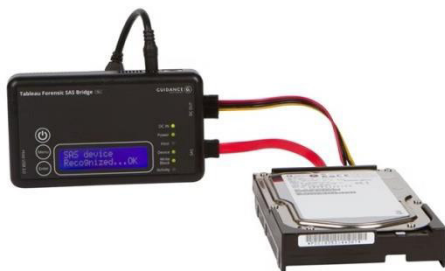
Fig 3 : Write-blocker machine prevents the evidence integrity
