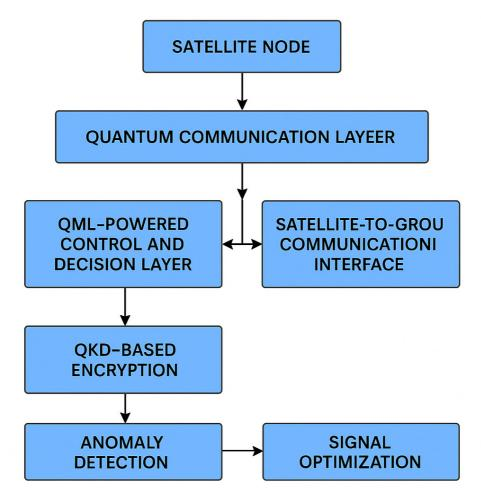
Figure 1:QKD integration with adaptive satellite communication model.
