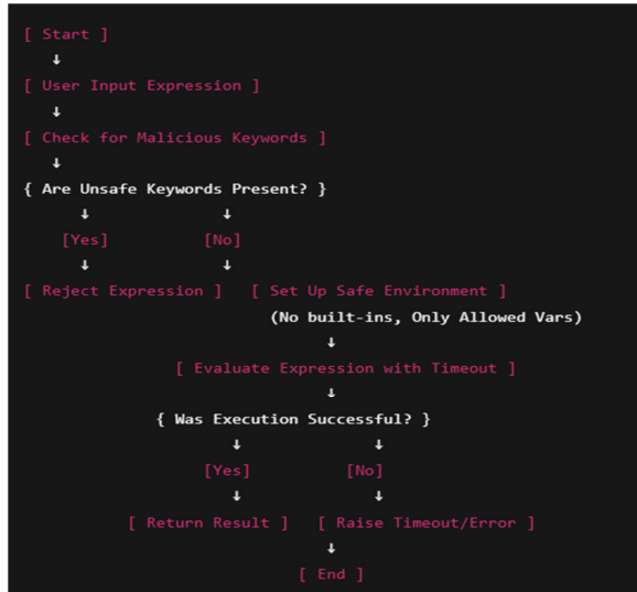
Figure 1: A Secure Execution Wrapper For Python's Eval() Function In Ai And Web Applications
