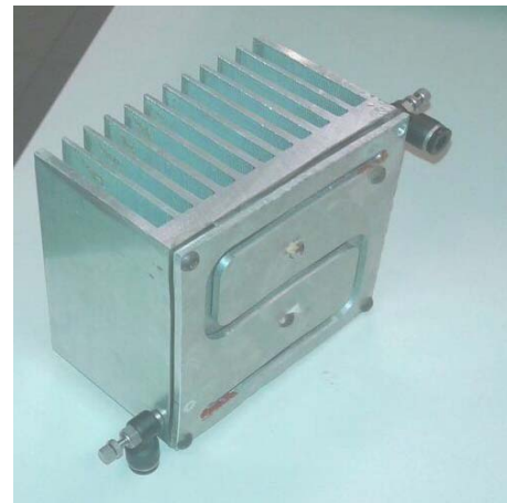
Fig.1 Aluminum finned cold plate used in this study
