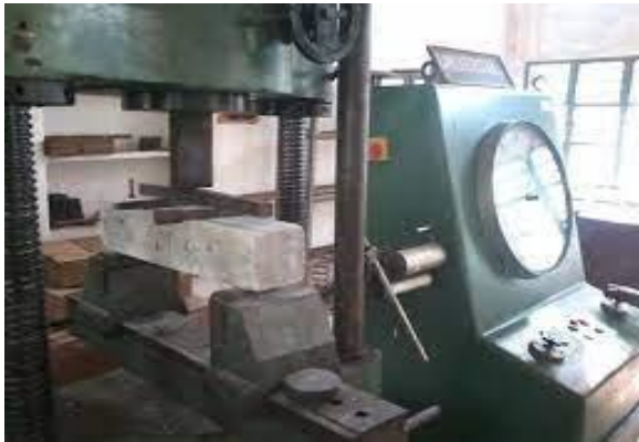
Fig. 3 Flexural strength test
