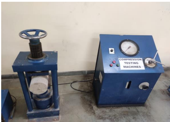
Fig. 4 Split tensile strength test
