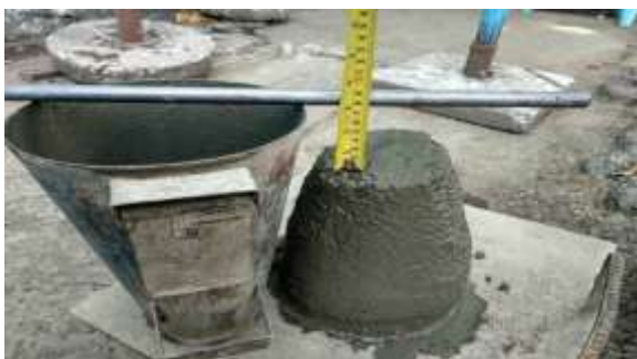
Fig. 1 Concrete slump testing
