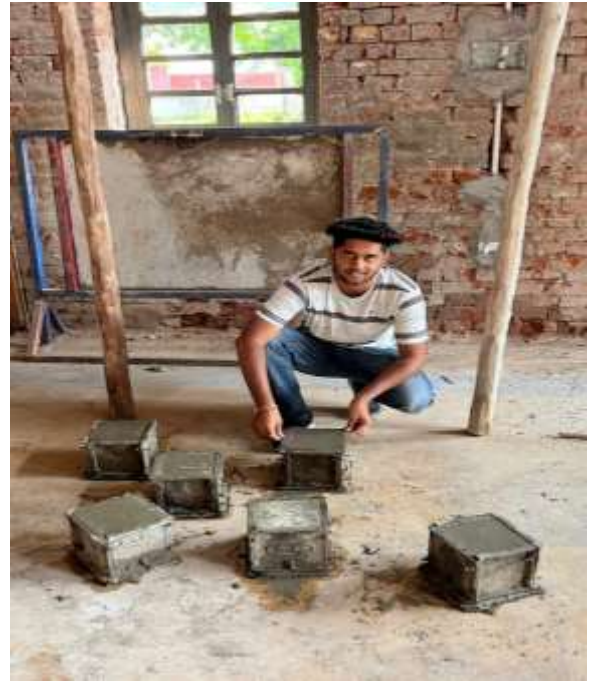
Fig. 4 Cube Casted for Experimental Work
