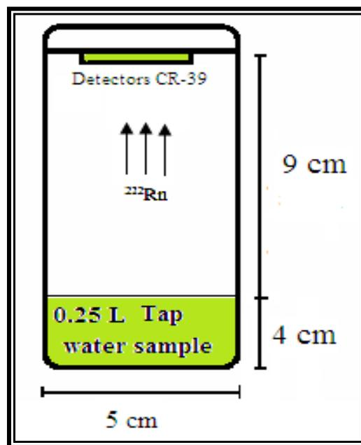
Fig. 2. Sealed-cup technique used for water samples
