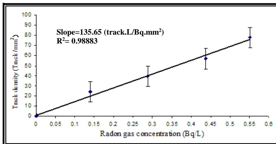
Fig. 3. Relation between radon gas concentration and track density in standard water samples
