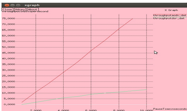
Fig. 8. Throughput of AODV and DSR for Six Nodes
