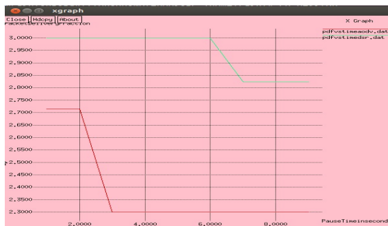
Fig. 9. Packet Delivery Fraction of AODV and DSR for Six Nodes
