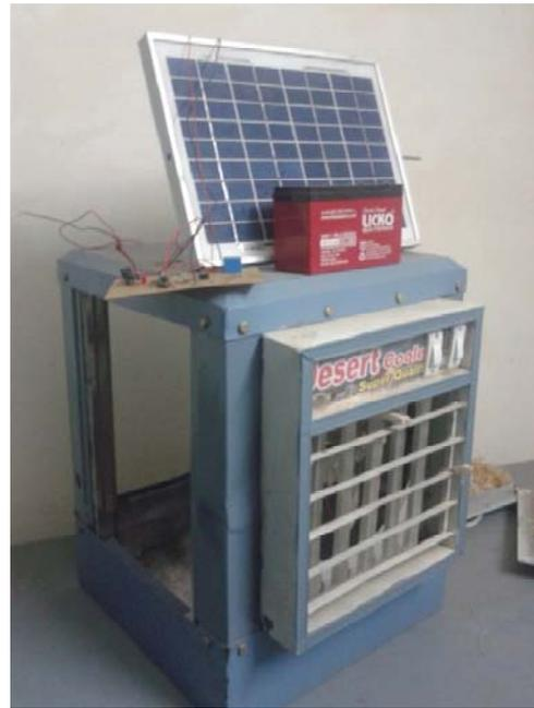
Fig.6 Solar Cooler
