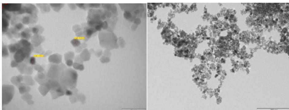
Fig. 4 TEM image of synthesized TiO<sub>2</sub> nanoparticles
