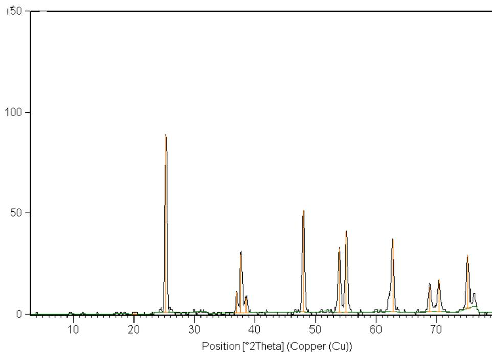
Fig. 2 XRD powder pattern of synthesized  $\text{TiO}_2$  by Sol-Gel
