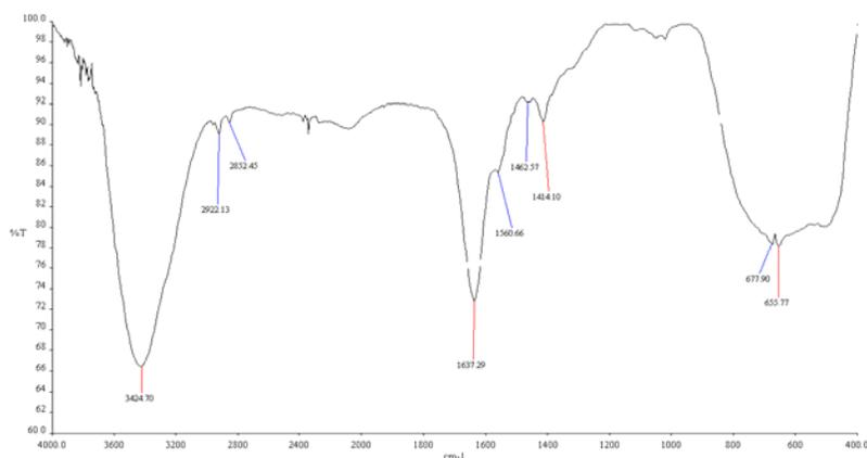
Fig. 3: FTIR spectra of synthesized TiO<sub>2</sub>
