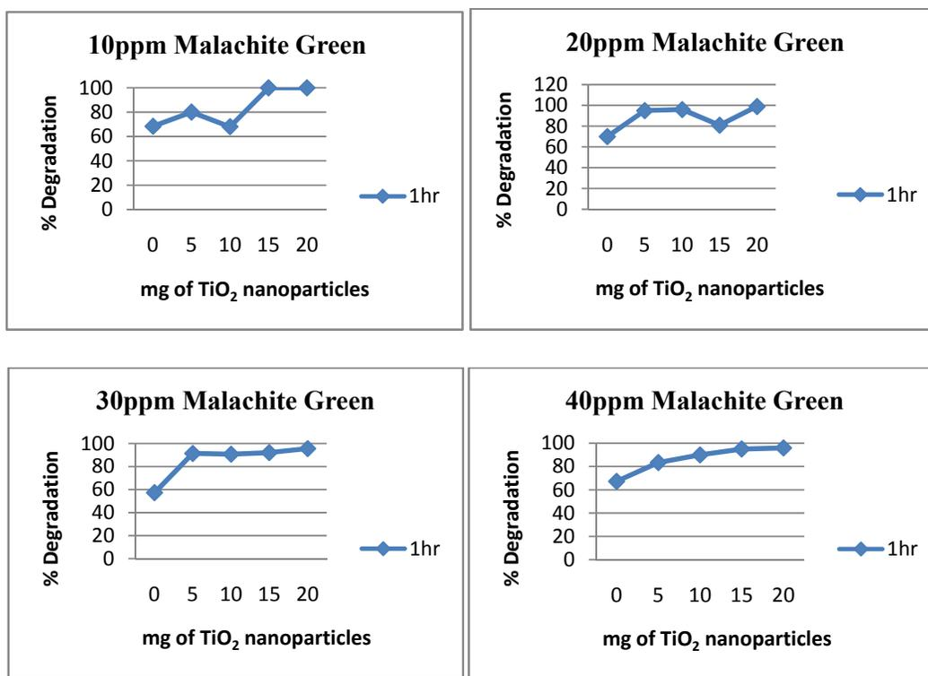
Fig.5 Degradation of Malachite Green by TiO<sub>2</sub> nanoparticles
