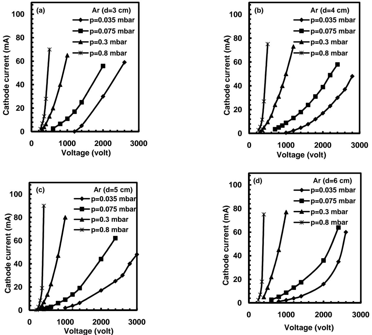
Fig.4: I-V characteristics of Ar discharge plasma at different value of gas pressure and inter-electrode spacing
