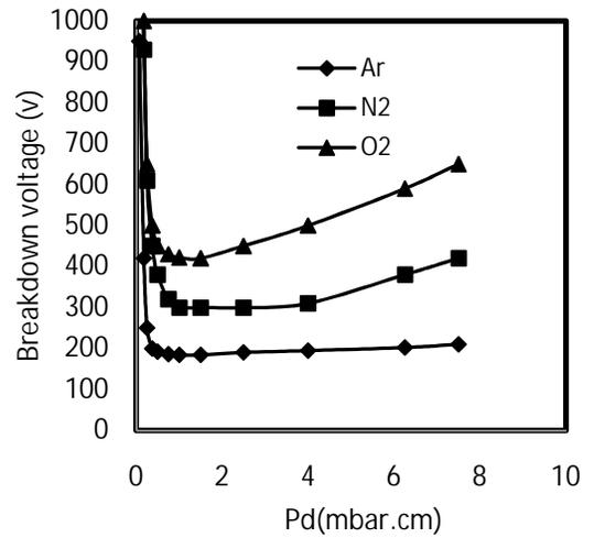
Fig.3: A plot of breakdown voltage as a function of pd with different gases for inter electrode spacing d=5cm.
