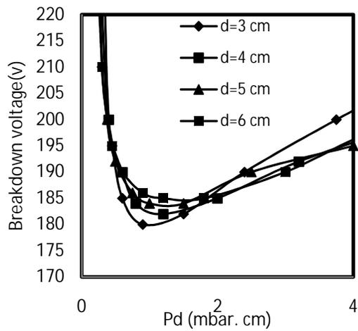
Fig.2: A plot of breakdown voltage of Ar as a function of pd with different inter-electrode spacing
