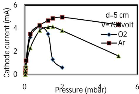
Fig.5:  $I$ - $P$  characteristics for different gases plasma with biasing voltage (700volt)
