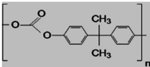
Fig. 1 Monomer structure of polycarbonate (PC)
