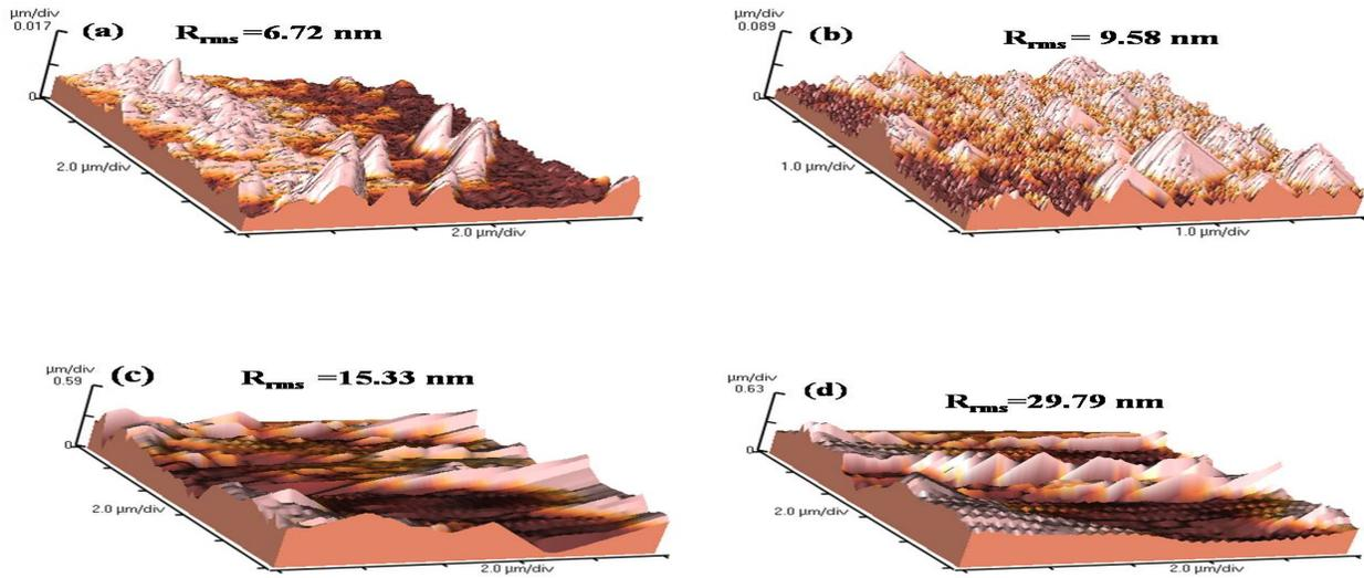
Fig.3. AFM images of Polycarbonate film with different plasma treatment time (a) untreated, (b) 10 min, (c) 30 min, and (d) 60 min.
