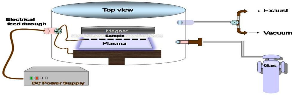
Fig. 2. Experimental set-up for plasma treatment system
