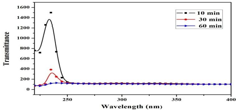
Fig. 5. UV-Visible spectrum for polycarbonate treated membrane for different irradiation time (a) 10 min (b) 30 min (c) 60 min.
