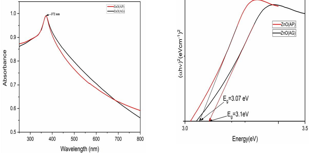
Fig. 3: Optical Spectra (a) Absorbance (b) Tauc plot for ZnO np's (AP & AG extract)
