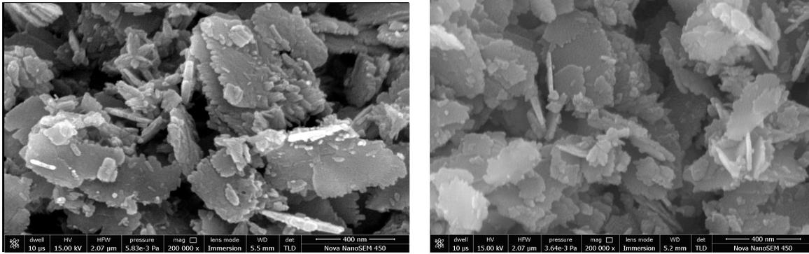
Fig. 1: Micrograph of ZnO np's of (a) AP (b) AG extract
