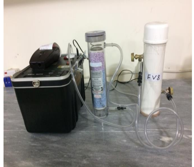
Fig. 2. Measuring radon concentration of soil samples in the Lab by RAD-7.
