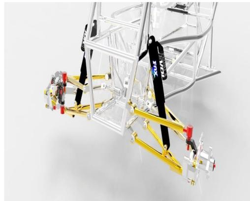
Fig. 6. Double Wishbone suspension system
