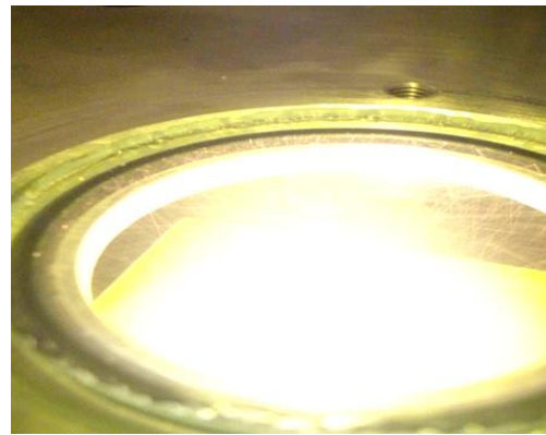
Fig. (2-d) The plasma generation due to the laser etching of TiO 2
