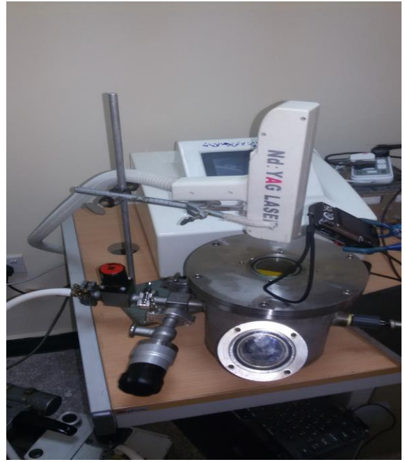
Fig. (4) The system which is used to generate the required plasma from the etching of TiO 2 nano disk by Nd:YAG laser pulses (1064 nm, 700 mj)
